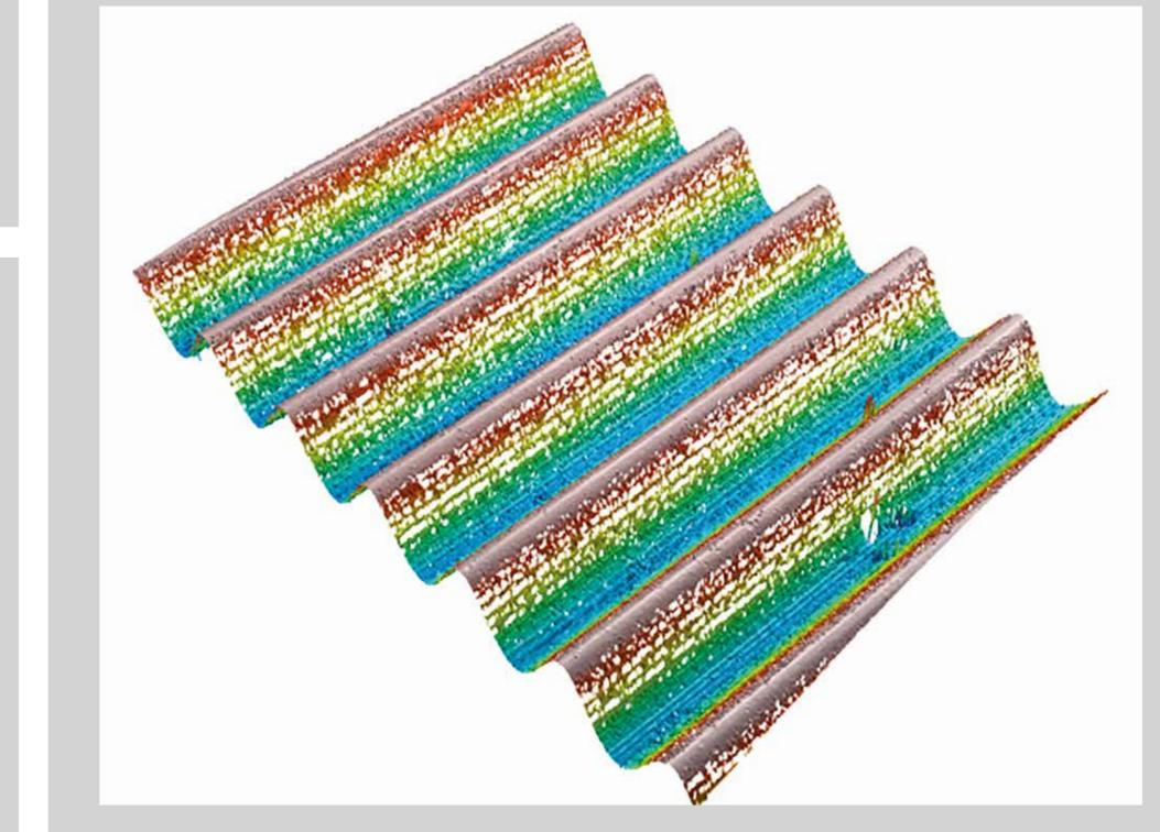
Roughness standard sample with Ra 3 μm. SineCopper pattern on glass substrate. Copperstructure measured with highest accuracy incylinders with 10 μm height. Although
