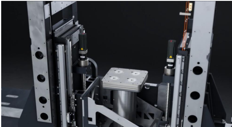
Up to 60 \mu\text{m} – 90 \mu\text{m} thermally induced expansion of piston
